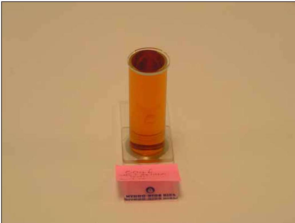
Figure 12. The phytoplankton in a 50 ml seawater sub-sample fixed with Lugol's iodine are allowed to settle onto the base plate of a settling chamber for a period of more than 20 hours before analysis.
