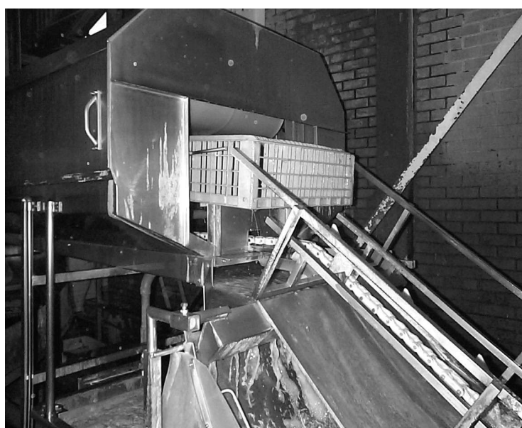
Figure 7: Crates entering main wash booth. The run down screen is visible in the lower part of the photograph; some fouling is evident.
