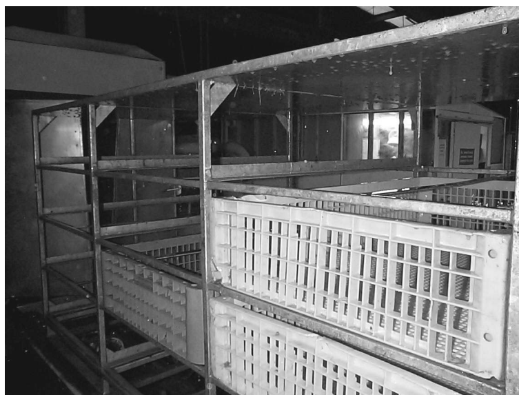
Figure 8: Washed crates stacked in steel transport frames (modules). These frames (modules) are washed separately in a batch wise fashion in large booths using sprays of recirculated water. Wash water can be seen dripping off the top surfaces of the module.
