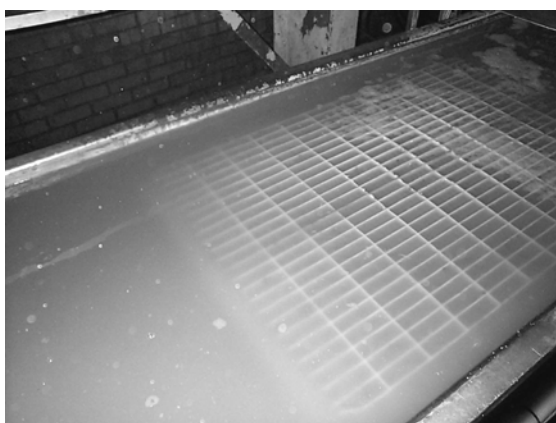
Figure 6: The main soak tank with crates passing through submerged. The length of these tanks can vary but typically they equate to 5-10 crate lengths. Plant speed will affect the actual residence time but around a minute would be usual.
