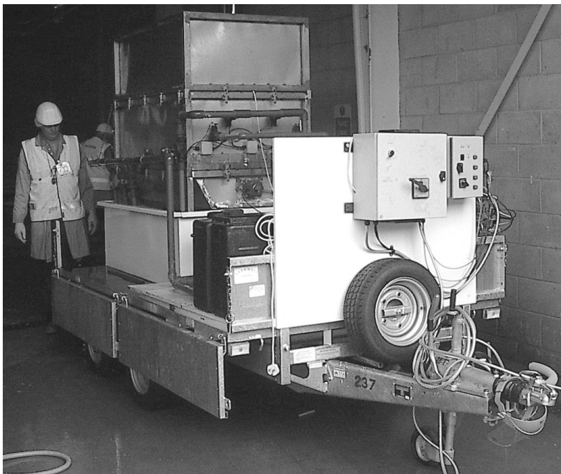
Figure 1: mobile crate washing rig used in factory based trials.
