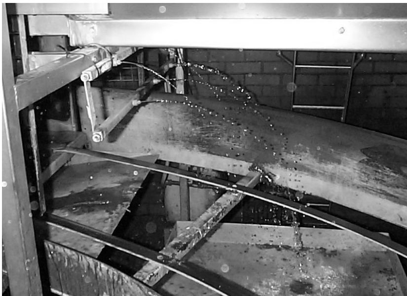
Figure 11: The continuous application of disinfectant in this example is clearly wasteful as well as being inadequate from a very poor jet. However, this is typical of many units but it still adds to the awarded HAS score. Some crate wash facilities have no disinfection system.
