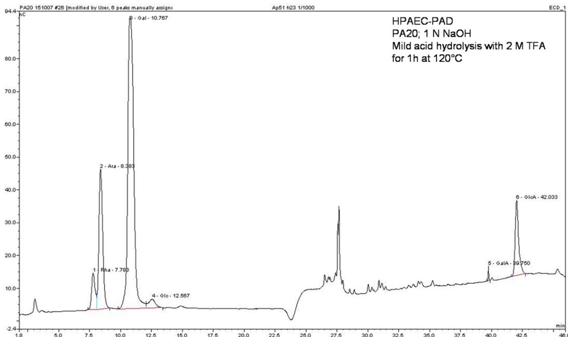
**Figure 7.** Sugar analysis of the AP51 polysaccharide by HPAEC-PAD using a Dionex PA20 column. AP51 contains rhamnose (Rha), arabinose (Ara), galactose (Gal) and glucuronic acid (GlcA) residues.
