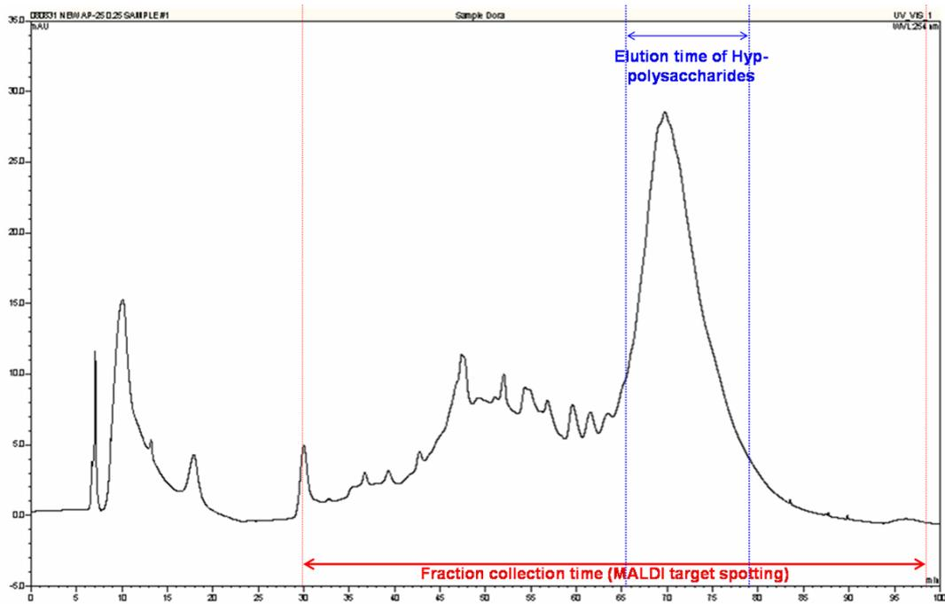
**Figure 9: UV chromatogram (at 254 nm) obtained by Normal Phase-Liquid Chromatography (NP-LC) of AP51 polysaccharide. The chromatogram shows the elution time of Hyp-polysaccharides.**
