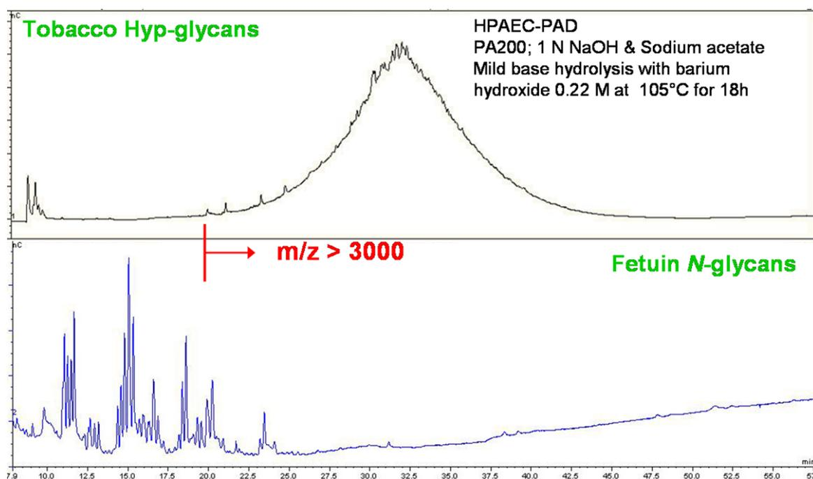
**Figure 8:** HPAEC-PAD analysis of AP51 polysaccharide using a Dionex PA200 column. These data indicate that the Hyp-linked glycans are extremely heterogeneous.
