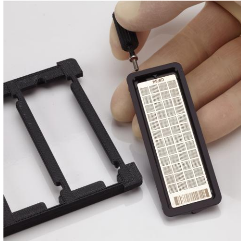
FIGURE 9 OPENARRAY HIGH THROUGHPUT PCR PLATFORM (obtained from http://www.lifetechnologies.com )
