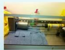
Fig. 1d. A miniature cheese press as produced to solve the high pressure required for pressing of Cheddar & Caerphilly cheese.
