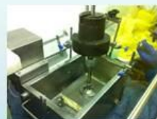
Fig. 1c. Apparatus for cheddar making mimicking the churning of the curd during traditional cheddar process.
