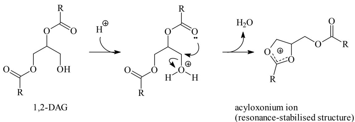
Figure 13. Formation of acyloxonium ion from 1,2-DAG
