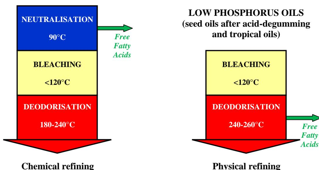
Figure 6. Overview of the main processes of edible oil refining
