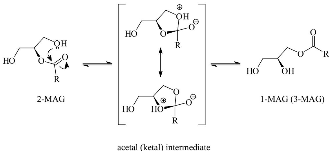
Figure 10. Mechanism of acyl migration in MAG
