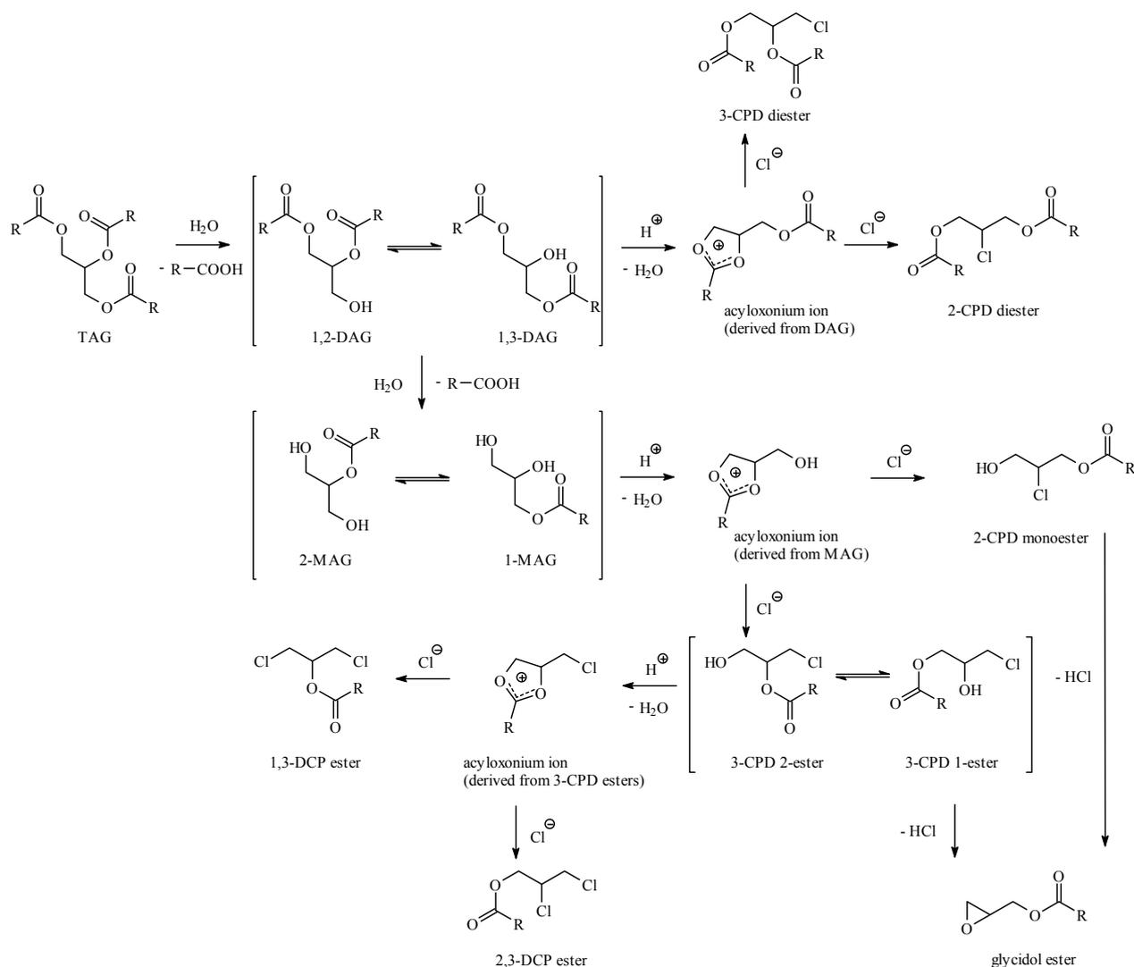
Figure 27. Proposed mechanisms of CPD esters, DCP esters and glycidol esters formation
