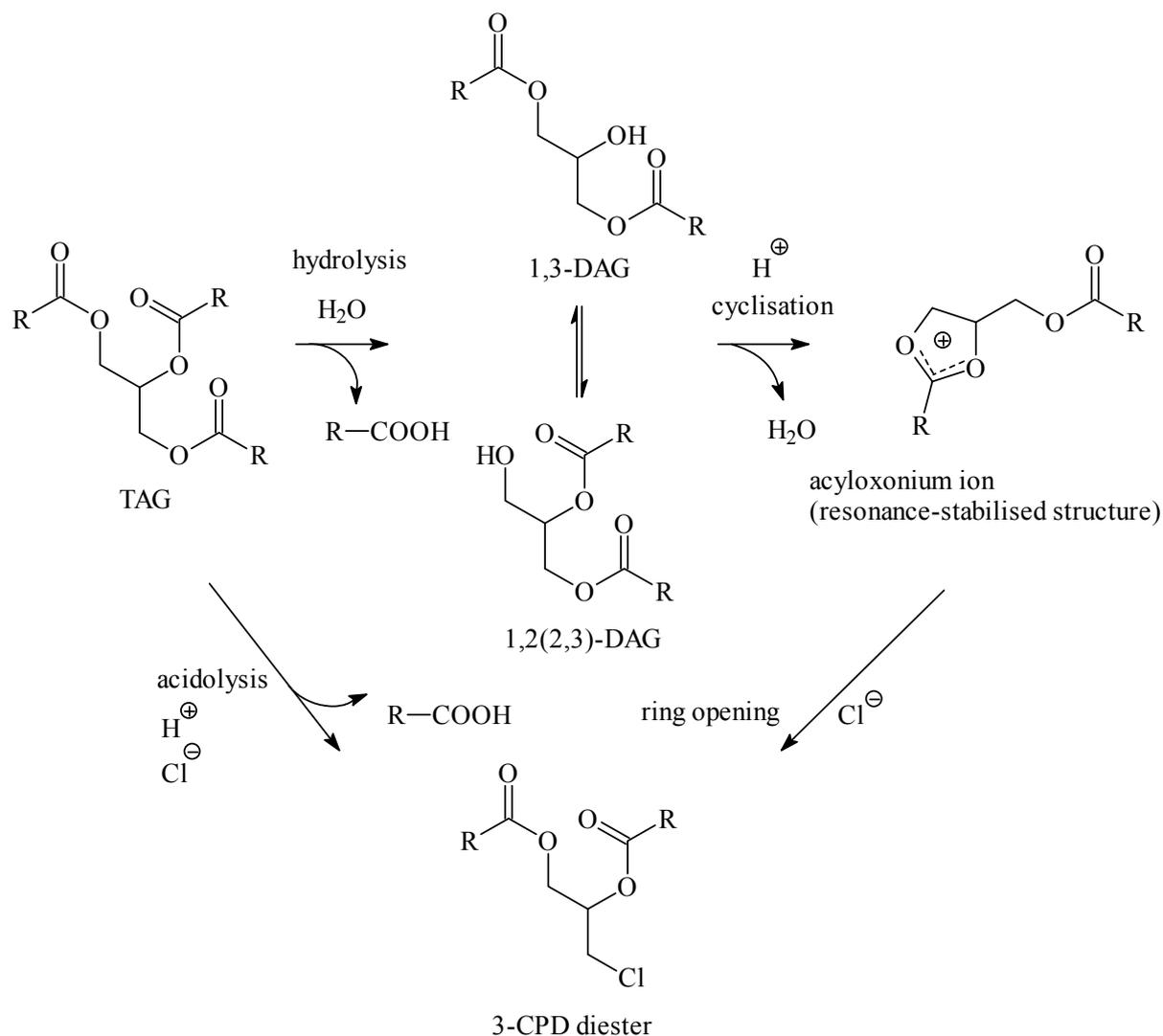
Figure 12. Formation of 3-CPD diesters from TAG *via* DAG (adapted from references [93] and [94])
