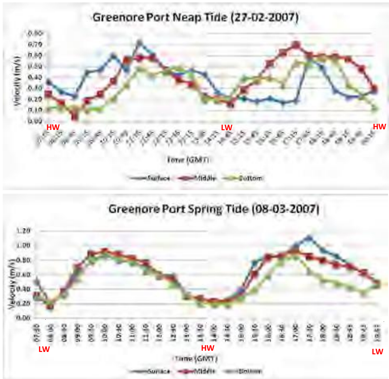
Figure 3.4: Tidal velocity (knots) over spring and neap tide at Greenore, Carlingford Lough (Source: Hydrographic Surveys Ltd., 2007).
