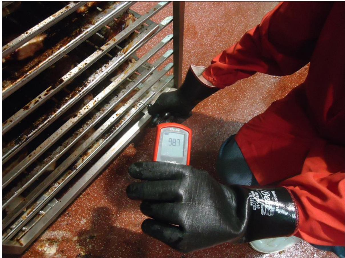
Figure 22 Manual temperature checking of thermally-processed meats using a temperature probe
