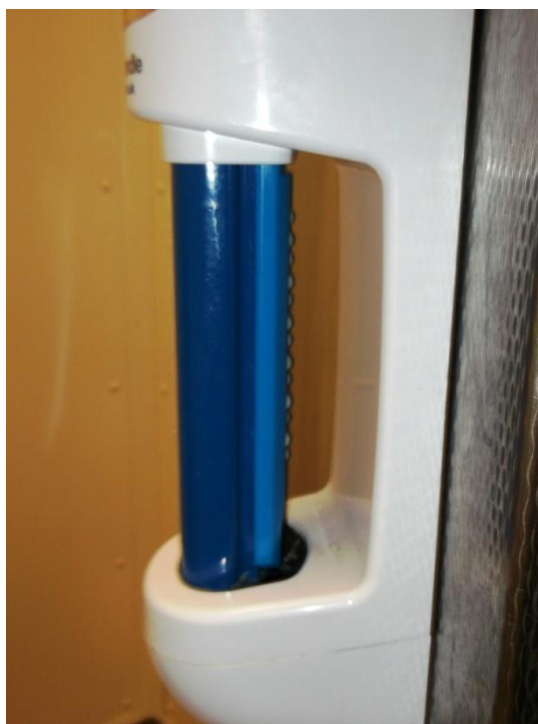
Figure 26 A door handle that dispensed alcohol onto workers' hands
