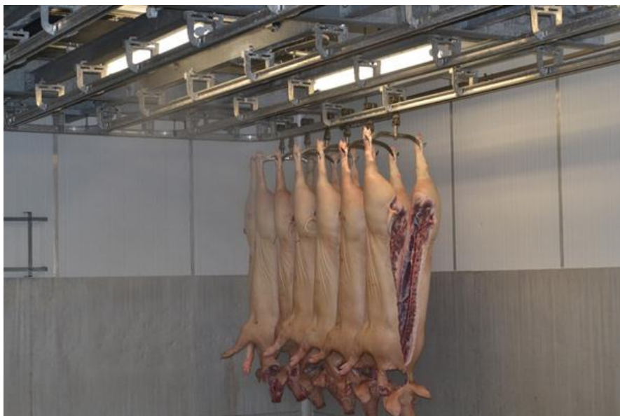
Figure 1 Heat removal from split pig carcasses after slaughter and dressing (processing to remove organs and inedible parts of the carcass)
