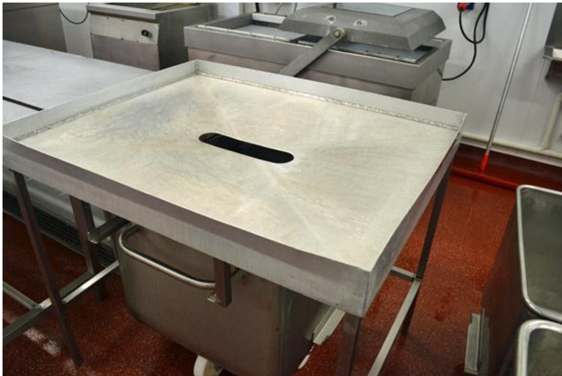
Figure 9 A self-draining work table used for the removal and disposal of elastic mesh and cook bag from the hams
