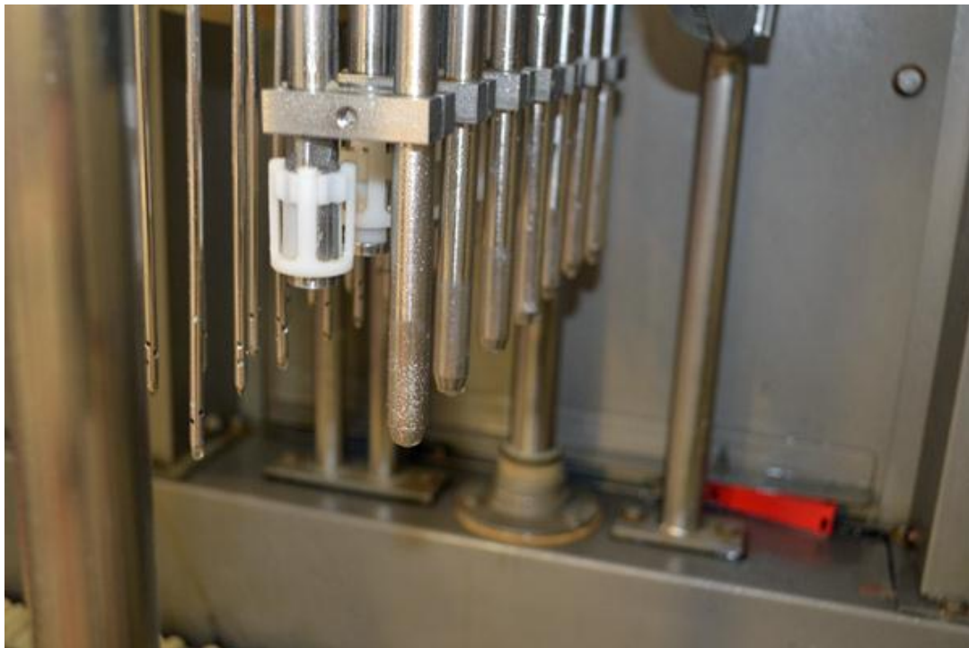
Figure 3 A set of injection needles used to transport brine under pressure into the centre of a pre-boned ham
