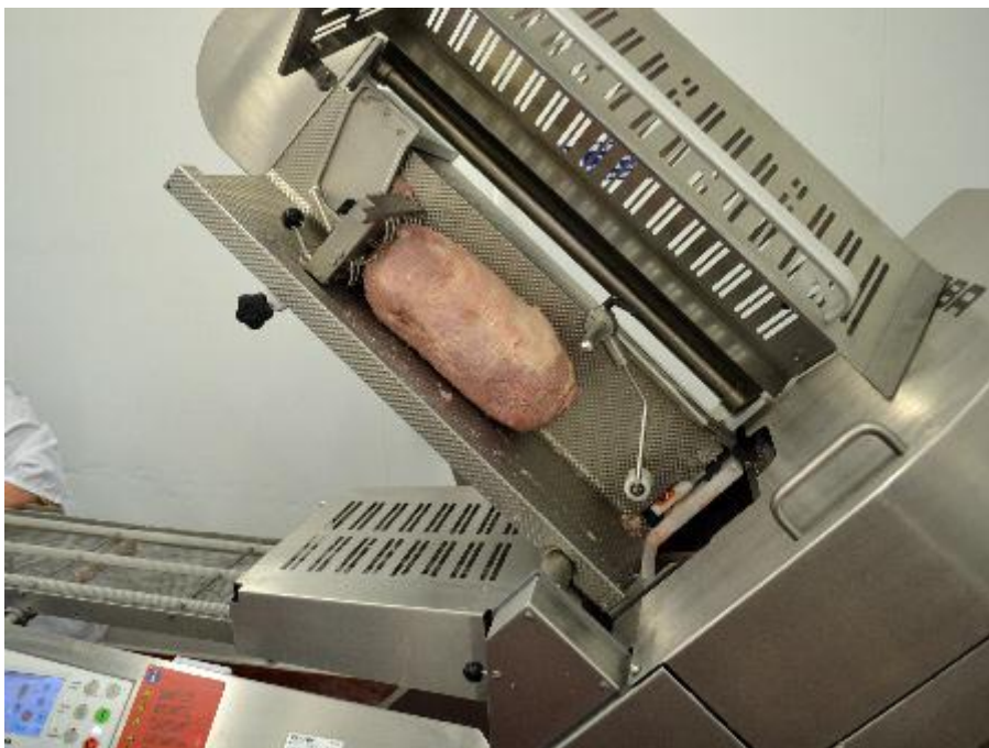
Figure 11 A log of ham being loaded into an automated slicer
