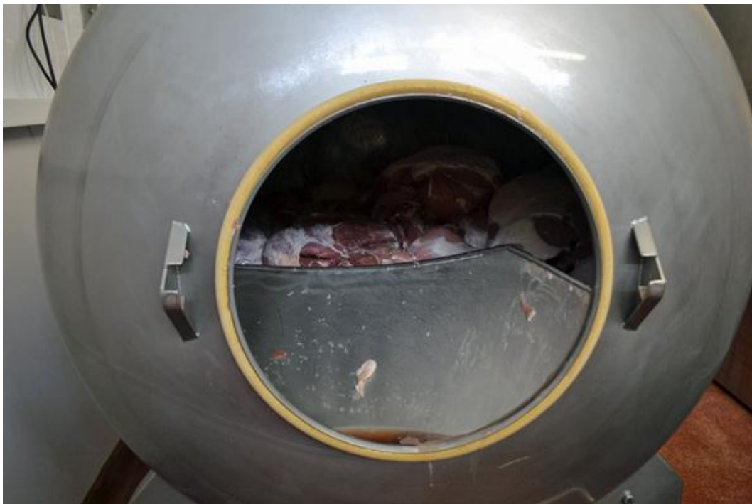
Figure 5 Hams after tumbling inside a rotating baffled drum for 16 hours prior to unloading
