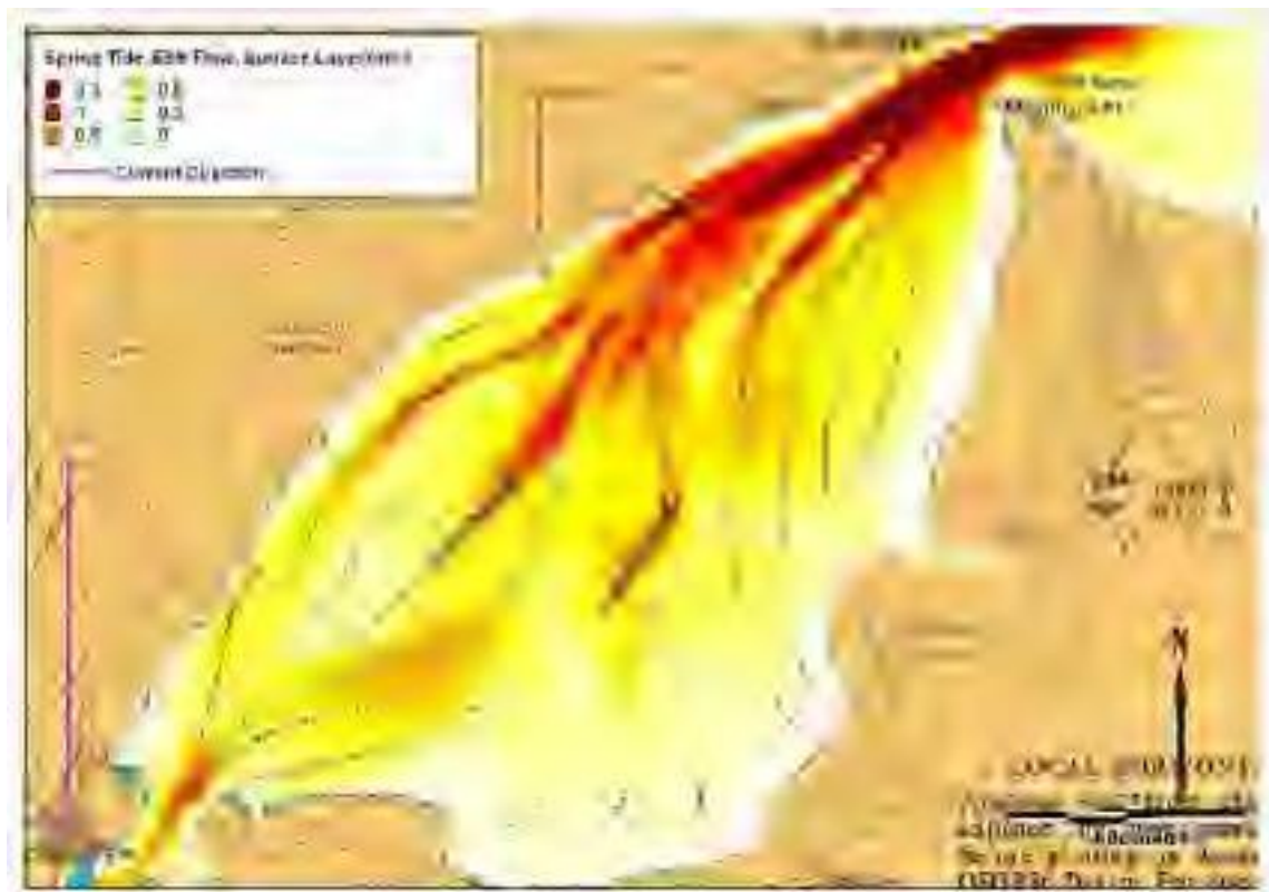
Figure 3.4: Surface current velocities and direction during a spring tide, ebb flow at 21:30:00 November 13 th 2008 (Source: Deltares Delft3D-FLOW).
