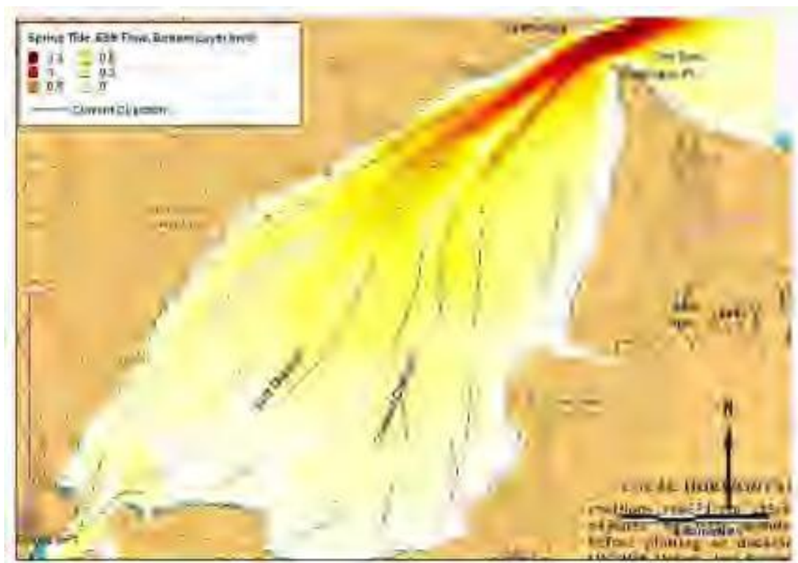
Figure 3.5: Bottom current velocities and direction during a spring tide, ebb flow at 21:30:00 November 13 th 2008 (Source: Deltares Delft3D-FLOW).
