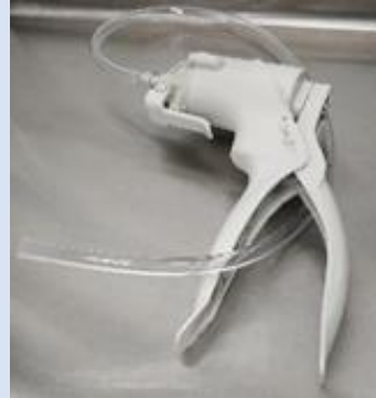
Water poured into the filter unit and filtered using a hand pump to collect bacteria on the filter paper.
