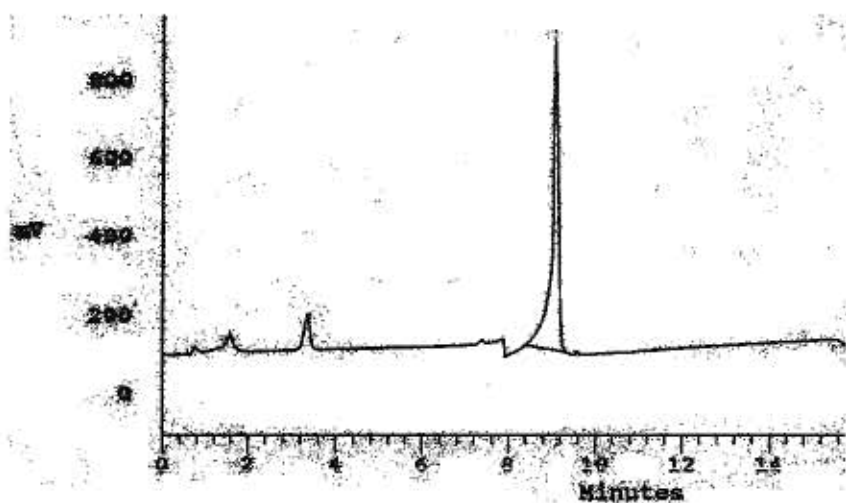
FIG.14 CHROMATOGRAPHIC SEPARATION OF TARTRATE IN DATEM HYDROLYSATE – NO CLEANUP
