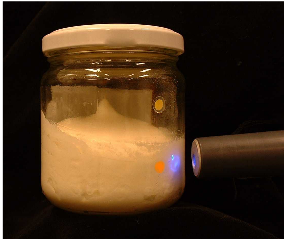
Figure 2. Set-up of the non-invasive oxygen determination. The yellow dot packed in the glass bottle contains the oxygen sensitive material.
