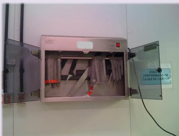
Photo 3. Open UV cabinet with tools inside
