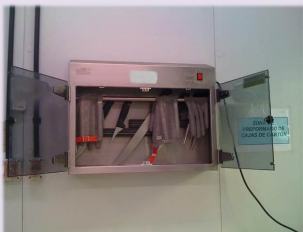
Photo 3. Open UV cabinet with tools inside
