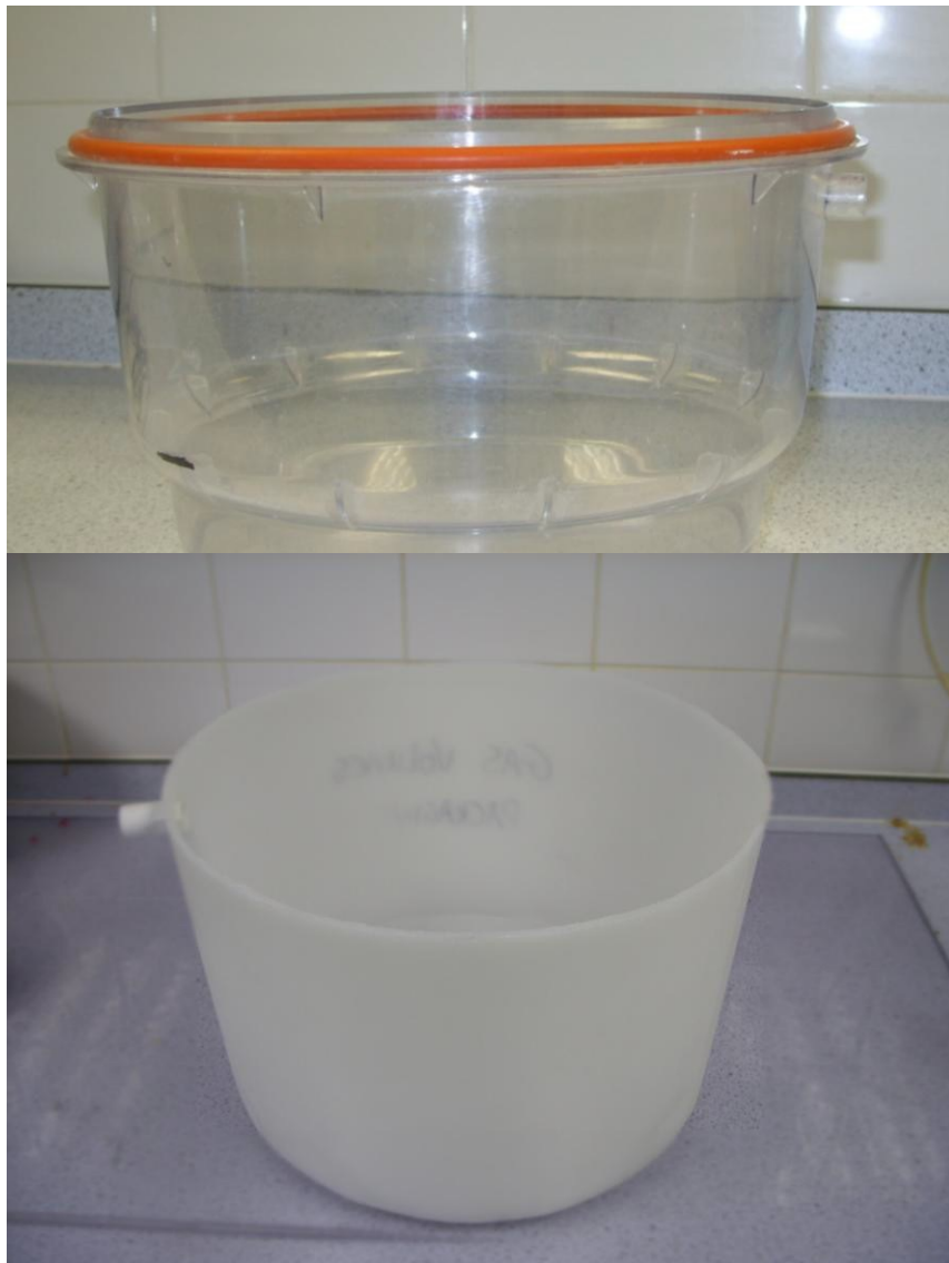
Figure 2. Photographs of containers with spouts used to measure the volumes of packs and poultry
