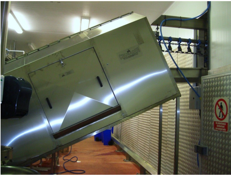
Figure A7 Photograph of side view of tunnel showing access panel
