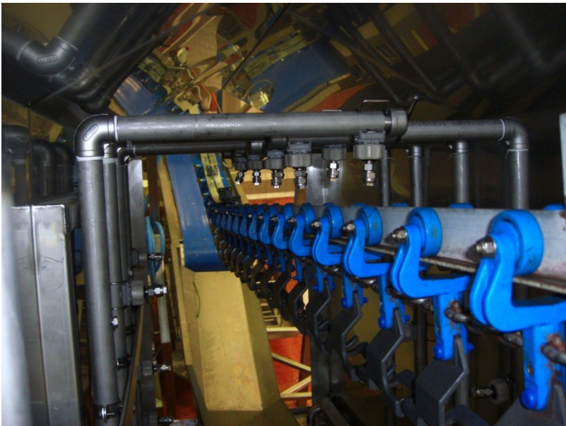
Figure A10 Spray nozzles located in the top of the tunnel for spraying liquid onto the top surface and into the body cavity of each chicken
