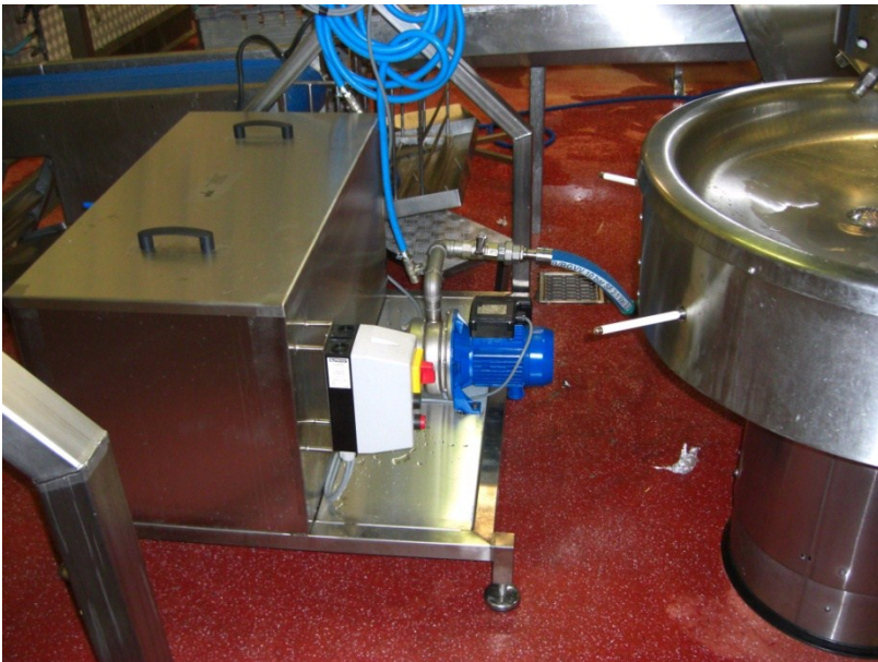
Figure A12 The tank and pump delivering liquid to the spray bars within the tunnel
