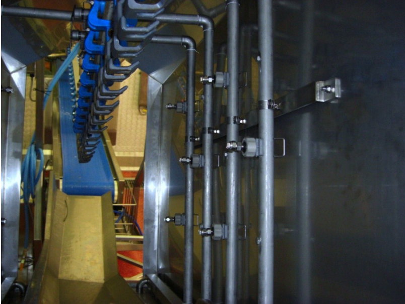
Figure A9 View inside tunnel showing spray bars on one side of the tunnel (a similar arrangement exists on the other side)
