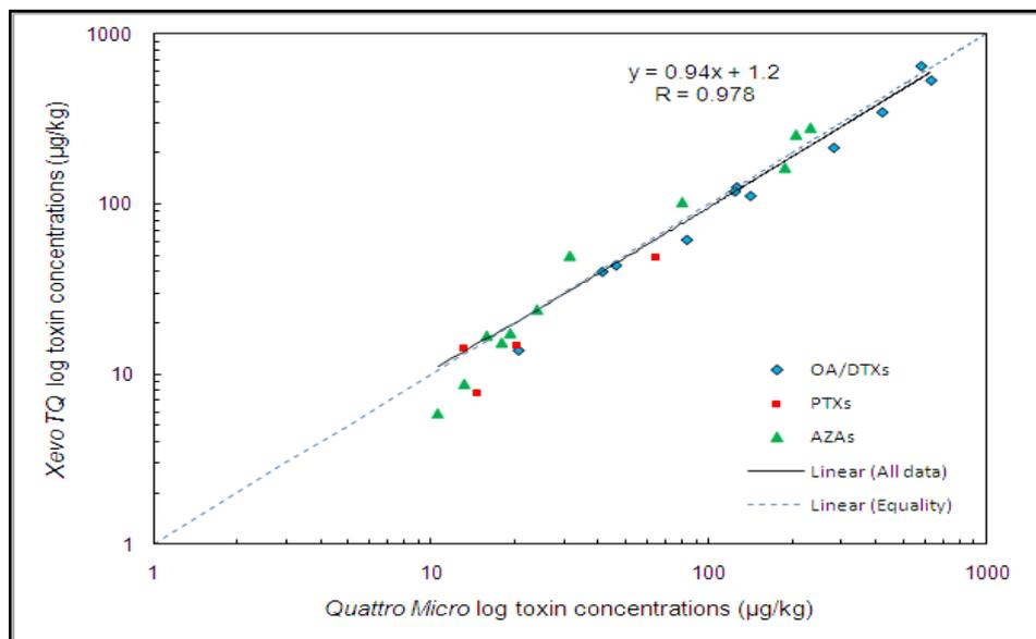
**Figure 18.** Comparison of log transformed toxin concentrations ( $\mu\text{g}/\text{kg}$ ) determined in naturally contaminated shellfish using the the *Quattro Micro* and *Xevo TQ* LC-MS/MS instruments, showing 95% confidence limits and equality.
