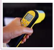
These types of probe are used for testing cold surface temperatures of food when delivered or in fridges and freezers.
