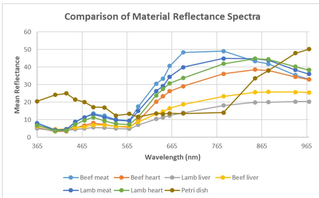
Figure 2. Typical VL4 generated reflectance spectra for ground beef meat and associated ground offal/meat materials
